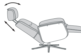
Manual Height and Angle Adjustable Headrest
